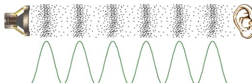
There are two important parameters of the sound: one is “frequency” value, the other is “amplitude” value. Knowing these two values of a sound signal provides us important information about that signal. The frequency of sound does not change with distance to the source of sound whereas its amplitude increases or decreases while getting closer to or farther away from the source.
