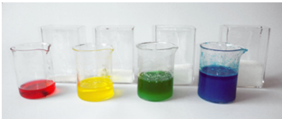
Figure 1: Coloured sugar solutions at various densities (concentrations)
